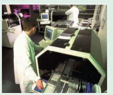
Automated screen printing of solder paste ensures precise component alignment.
