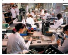
Soldering is either by hand or automated wave soldering as appropriate to the board complexity and batch size.
